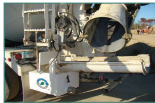
Chute washout box
